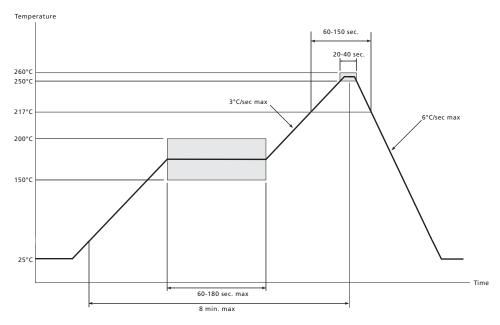
Figure 6-1: Maximum Pb-free Solder Reflow Profile
