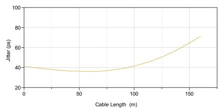
Figure 2-2: Jitter vs. Cable Length (1485 Mb/s)
