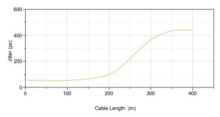
Figure 2-1: Jitter vs. Cable Length (270 Mb/s)
