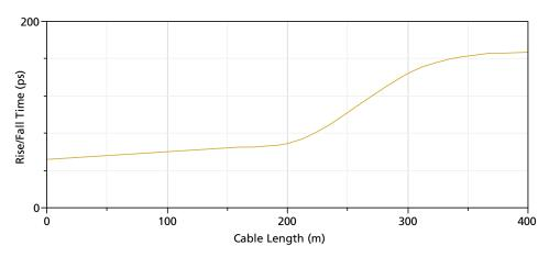
Figure 3-3: Typical Rise/Fall Time for 270Mb/s Data Rate (VCC=3.3V, room temperature, 800mV launch swing)
