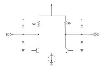
Figure 5-3: Output Circuit
