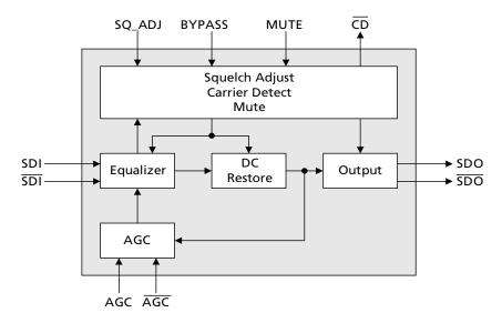
Figure 3-1: GS1674 Functional Block Diagram
