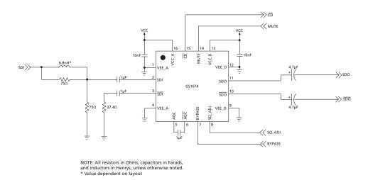
Figure 4-1: GS1674 Typical Application Circuit
