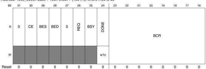
Address: 4000\_8000h base + 108h offset +  $(16d \times i)$ , where i=0d to 3d
