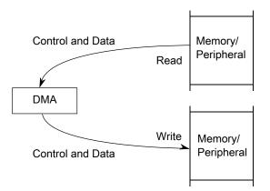
Figure 19-2. Dual-Address Transfer
