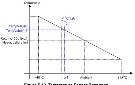
Figure 5-12. Temperature Sensor Response
