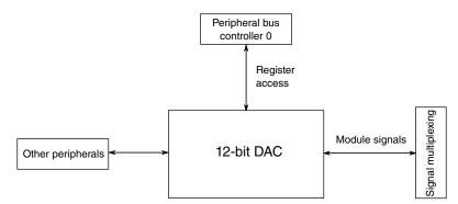
Figure 1-24. 12-bit DAC configuration
