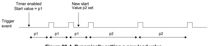
Figure 28-4. Dynamically setting a new load value
