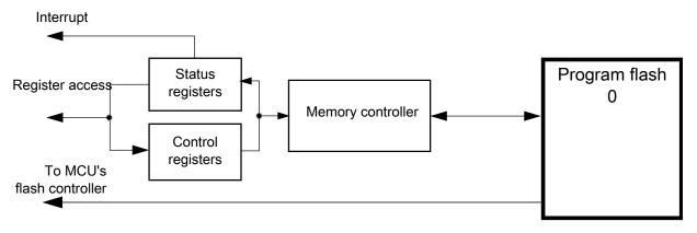
Figure 23-1. Flash Block Diagram
