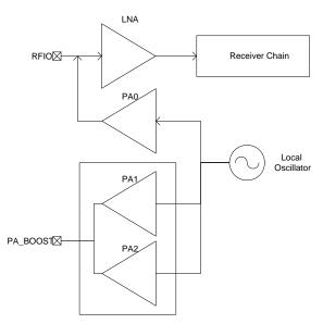
Figure 5-3. Transmitter Block Diagram
