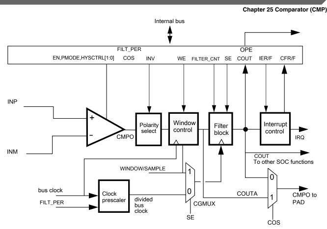
Figure 25-2. Comparator module block diagram
