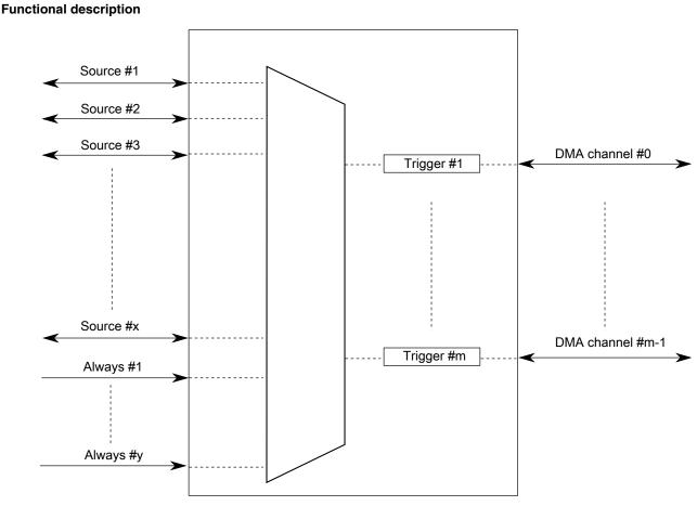
Figure 18-2. DMAMUX triggered channels
