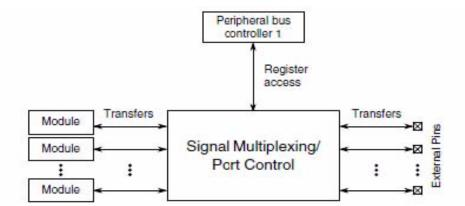
Figure 3-1. Signal Multiplexing Integration
