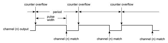
Figure 27-9. EPWM period and pulse width with ELSnB:ELSnA = 1:0
