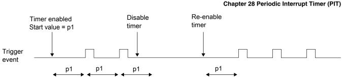
Figure 28-2. Stopping and starting a timer
