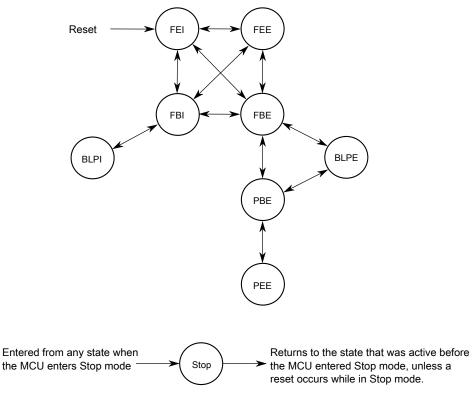
Figure 20-2. MCG mode state diagram
