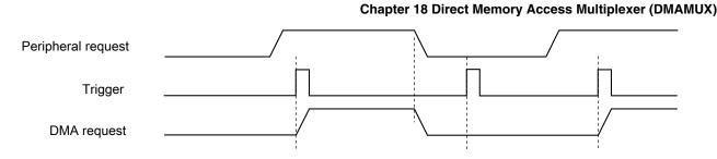
Figure 18-4. DMAMUX channel triggering: ignored trigger
