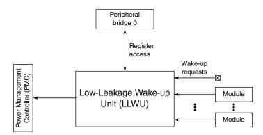
Figure 1-7. Low-Leakage Wake-up Unit configuration
