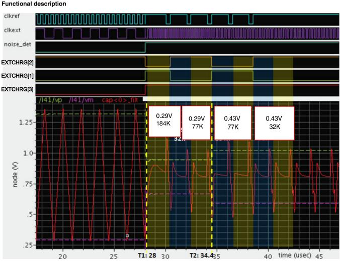
Figure 35-9. TSI noise detection mode waveform
