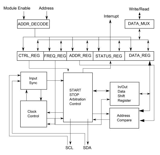
Figure 36-1. I2C Functional block diagram
