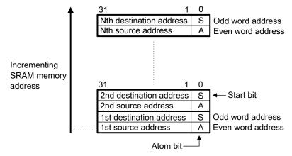
Figure 15-2. MTB execution trace storage format
