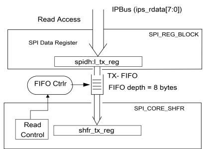
Figure 31-4. SPIH:L write side structural overview in FIFO mode
