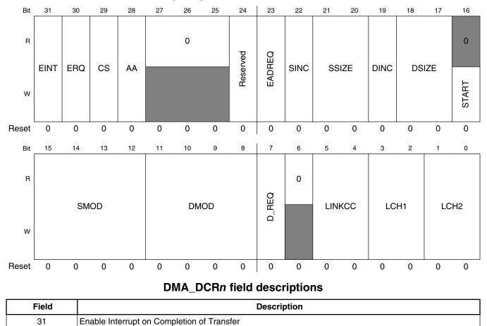
Address:  $4000_{8000h}$  base + 10Ch offset + (16d × i), where i=0d to 3d
