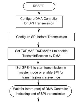
Figure 31-5. Basic Flow of SPI Transmission by DMA
