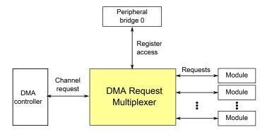
Figure 1-11. DMA request multiplexer configuration
