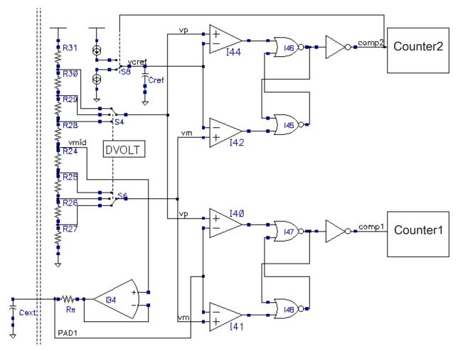
Figure 35-6. TSI circuit in noise detection mode
