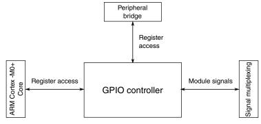
Figure 1-32. GPIO configuration
