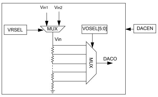
Figure 25-6. 6-bit DAC block diagram
