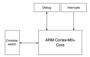
Figure 1-1. Core configuration
