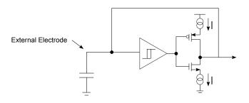
Figure 35-2. TSI electrode oscillator circuit
