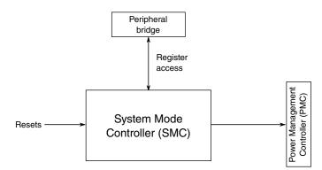
Figure 1-5. System mode controller configuration
