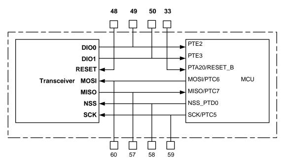
Figure 8-1. MKW01 Internal Interconnects Highlighting SPI Bus
