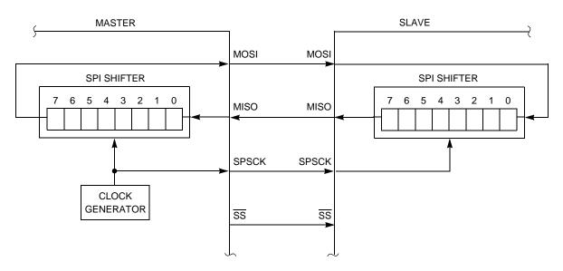
Figure 8-2. SPI System Block Diagram
