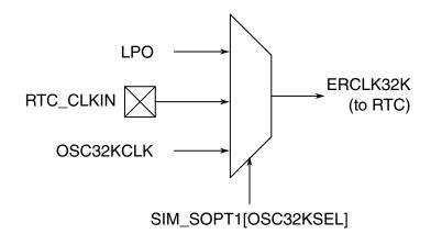
Figure 3-3. RTC clock generation
