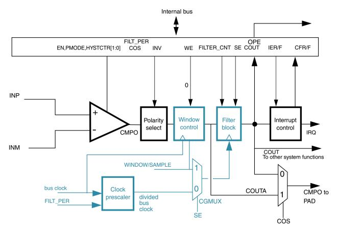
Figure 25-3. Comparator operation in Continuous mode
