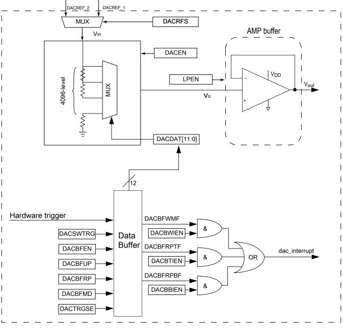
Figure 26-1. DAC block diagram
