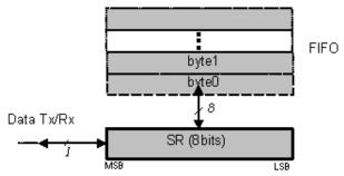
Figure 7-3. FIFO and Shift Register (SR)
