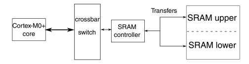
Figure 1-19. SRAM configuration
