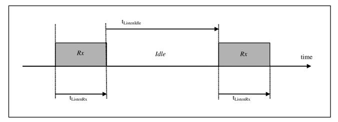
Figure 6-5. Listen Mode Sequence (no wanted signal is received)
