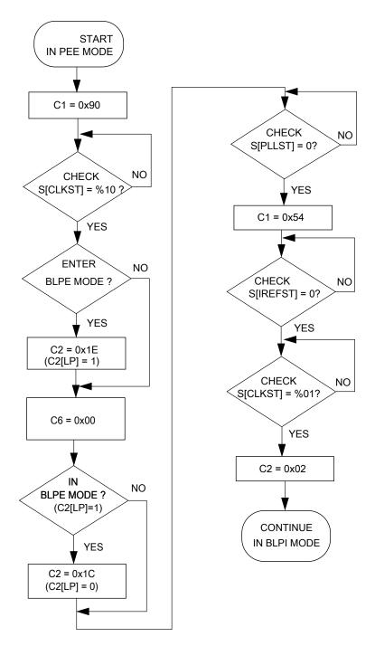
Figure 20-4. Flowchart of PEE to BLPI mode transition using an 4 MHz crystal
