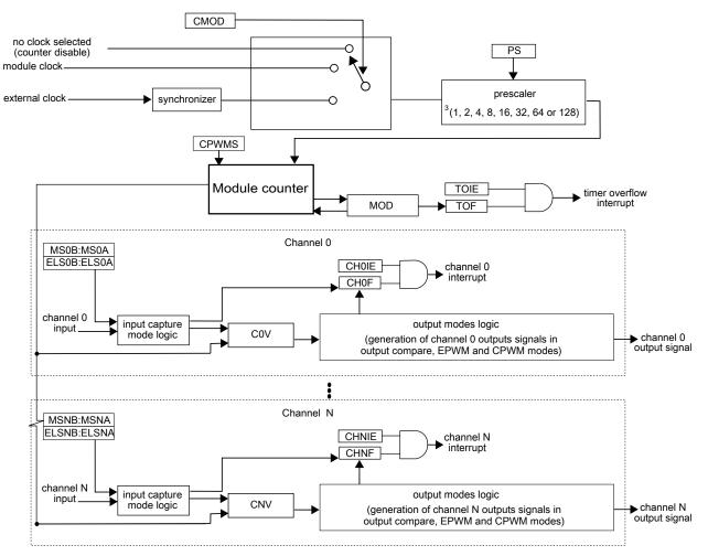
Figure 27-1. TPM block diagram
