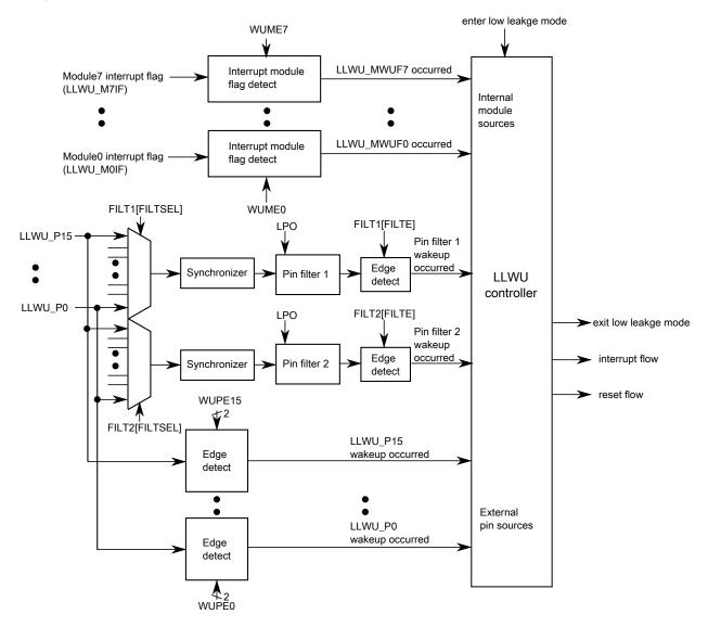
Figure 11-1. LLWU block diagram
