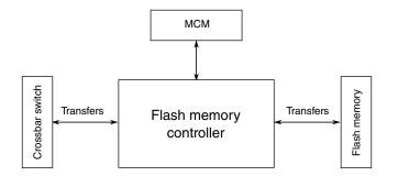
Figure 1-18. Flash memory controller configuration
