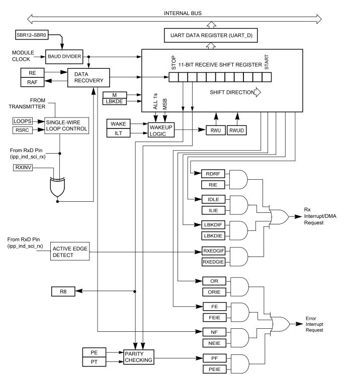
Figure 33-2. UART receiver block diagram
