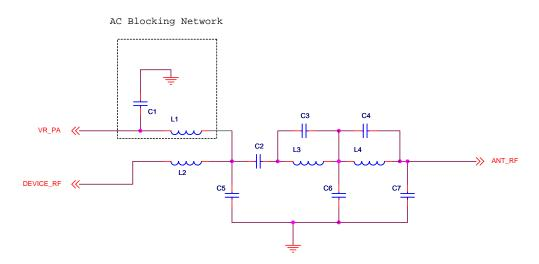
Figure 4-7. General RF Filter/Matching Network Topology
