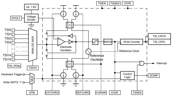
Figure 35-1. TSI module block diagram
