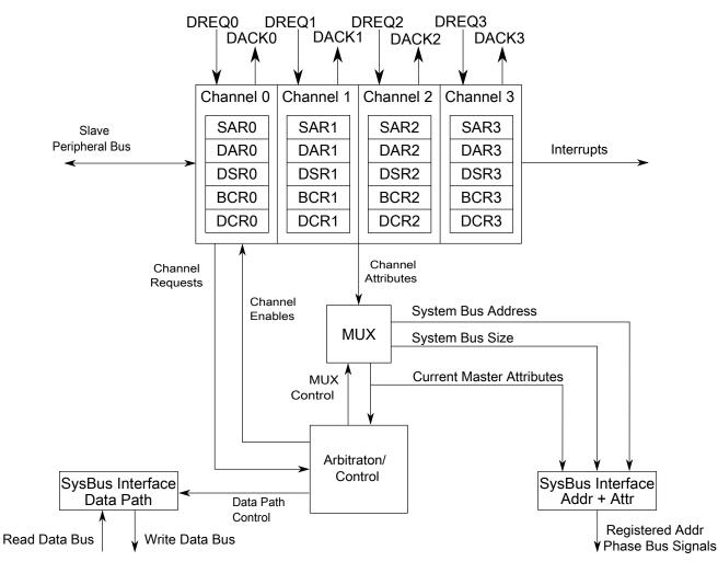
Figure 19-1. 4-Channel DMA Block Diagram
