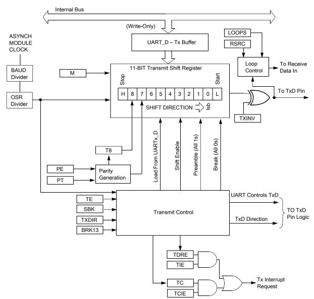
Figure 32-1. UART transmitter block diagram
