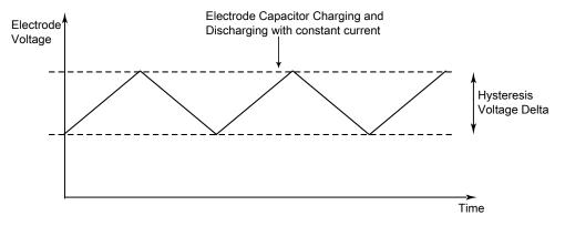
Figure 35-3. TSI electrode oscillator chart
