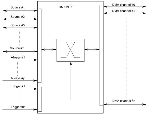
Figure 18-1. DMAMUX block diagram
