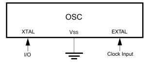
Figure 21-5. External Clock Connections
