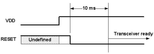
Figure 4-2. POR Timing Diagram
