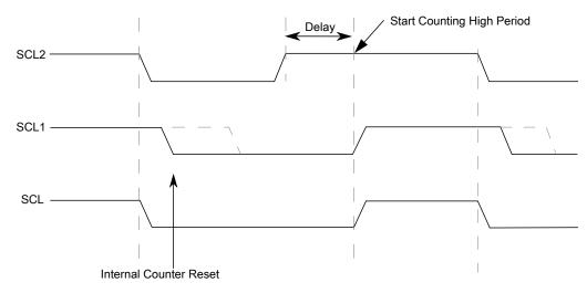
Figure 36-3. I2C clock synchronization
