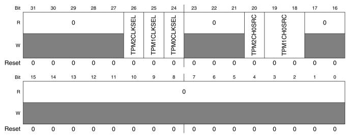
Address: 4004\_7000h base + 100Ch offset = 4004\_800Ch
