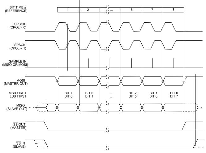
Figure 31-6. SPI clock formats (CPHA = 1)
