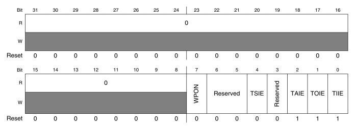
Address: 4003\_D000h base + 1Ch offset = 4003\_D01Ch
