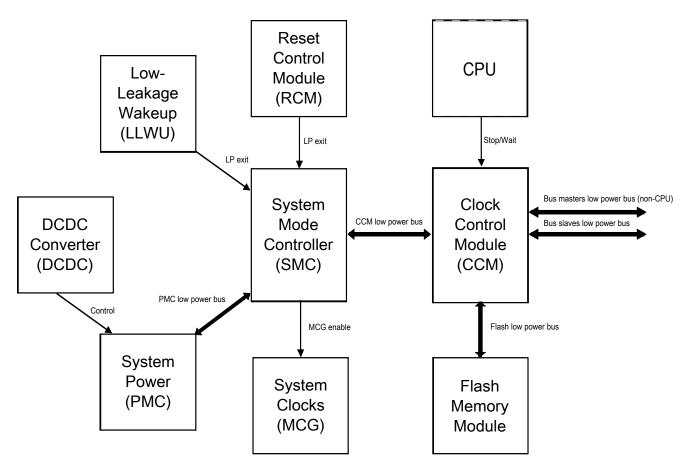
Figure 9-2. Low-power system components and connections
