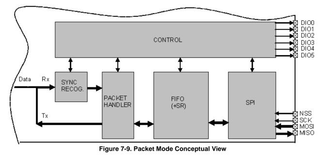
The Bit Synchronizer is automatically enabled in Packet mode.
