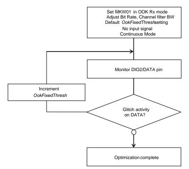
Figure 5-8. Floor Threshold Optimization
