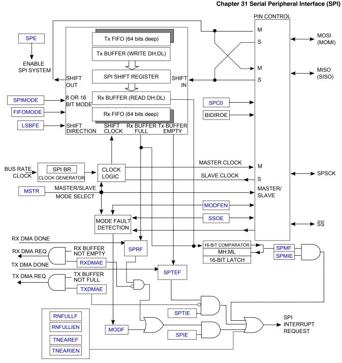
Figure 31-2. SPI Module Block Diagram with FIFO
