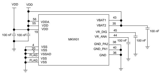
Figure 4-1. MKW01Z128 power supply connections
