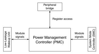
Figure 1-6. PMC configuration
