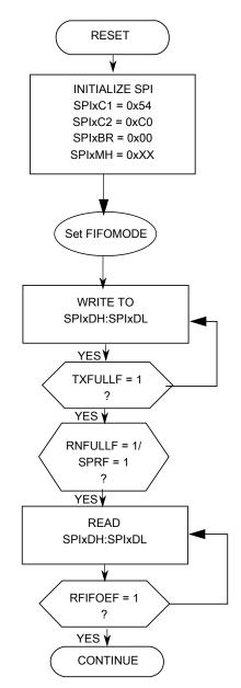
Figure 31-10. Initialization Flowchart Example for SPI Master Device in 16-bit Mode for FIFOMODE = 1
