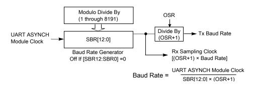
Figure 32-3. UART baud rate generation
