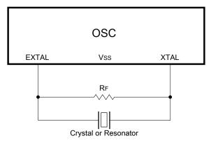
Figure 21-3. Crystal/Ceramic Resonator Connections - Connection 2
