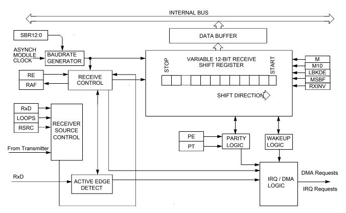
Figure 32-2. UART receiver block diagram
