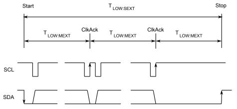
Figure 36-4. Timeout measurement intervals
