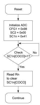
Figure 24-2. Initialization flowchart example
