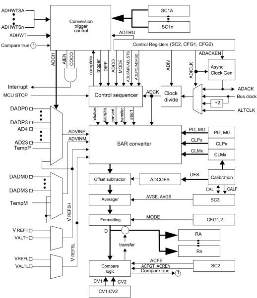
Figure 24-1. ADC block diagram
