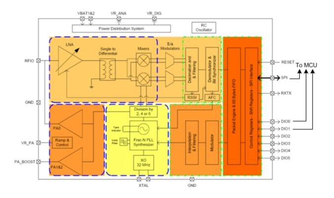
Figure 5-1. MKW01Z128 Transceiver Block Diagram
