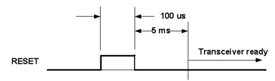
Figure 4-3. Manual Reset Timing Diagram
