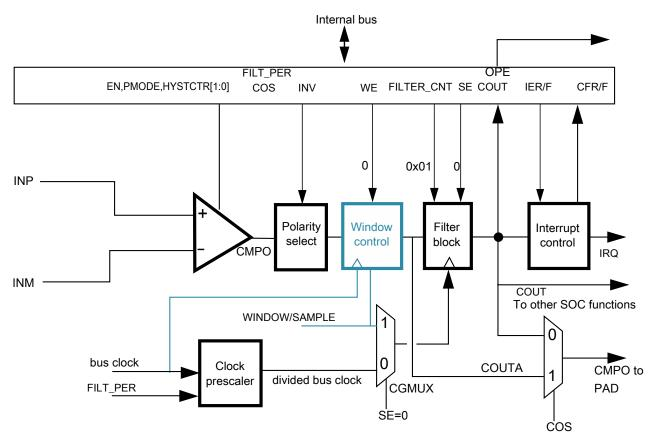
Figure 25-4. Sampled, Non-Filtered (# 3B): sampling interval internally derived
