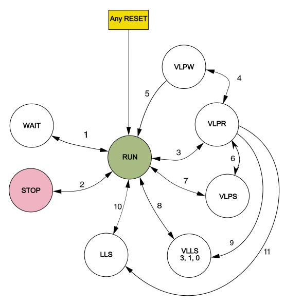
Figure 9-1. Power mode state diagram
