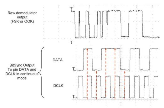
Figure 5-9. Bit Synchronizer Description
