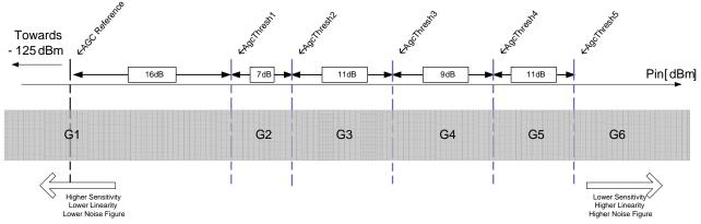
Figure 5-5. AGC Thresholds Settings
