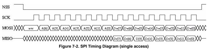
MOSI is generated by the master on the falling edge of SCK and is sampled by the slave (i.e. this SPI interface) on the rising edge of SCK. MISO is generated by the slave on the falling edge of SCK.
