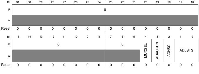
Address: 4003\_B000h base + Ch offset = 4003\_B00Ch
