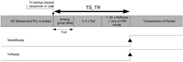
Figure 6-1. TX Startup, FSK and OOK
