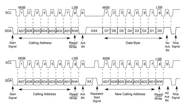
Figure 36-2. I2C bus transmission signals
