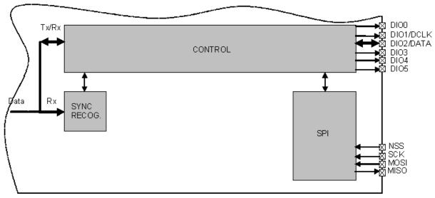
Figure 7-6. Continuous Mode Conceptual View
