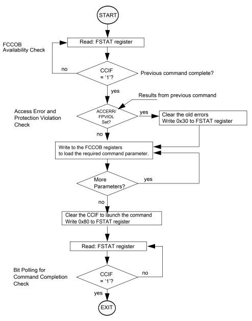
Figure 23-3. Generic flash command write sequence flowchart
