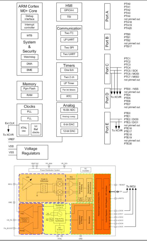
Figure 1-1. MKW01 system level block diagram
