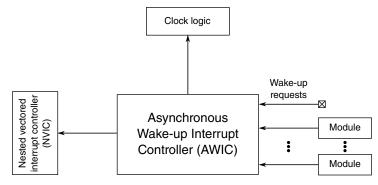
Figure 1-3. Asynchronous wake-up interrupt controller configuration
