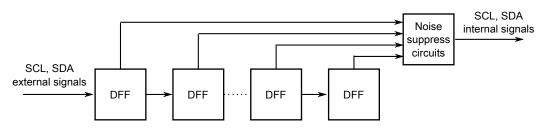
Figure 36-5. Programmable input glitch filter diagram
