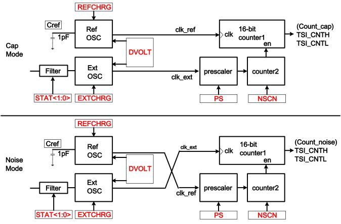
Figure 35-5. TSI noise detection mode block diagram
