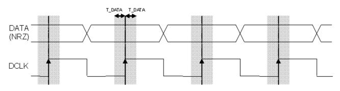
Figure 7-7. TX Processing in Continuous Mode
