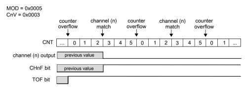
Figure 27-7. Example of the output compare mode when the match clears the channel output
