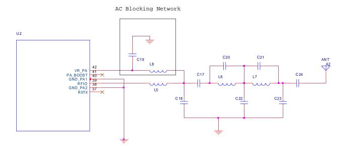
Figure 4-5. Single Port RF Schematic (+13dBm)
