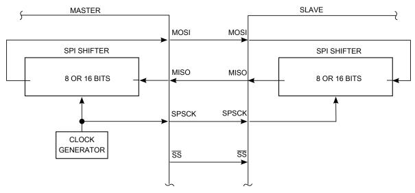
Figure 31-1. SPI system connections
